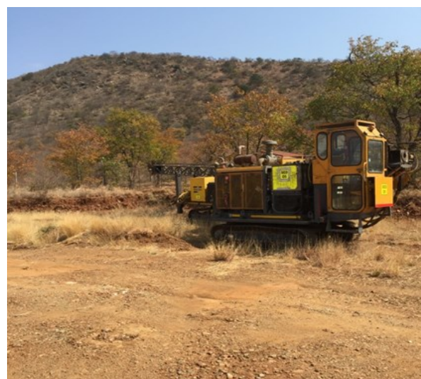
Positioning the drill rig at the Louwskop project prior to set up and commencement of diamond drilling.
